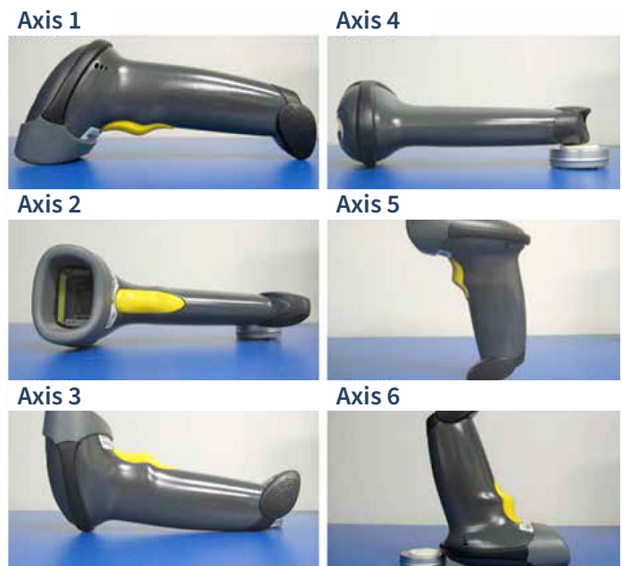
Figure 1. Hand-held scanner dropped in 6 axis during shock testing.
